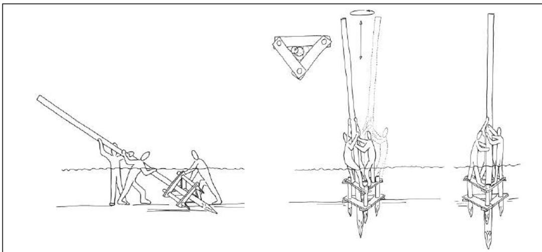
**Fig. 1 Schematic illustration of the Bronze Age method of installing wood piles over water (from Menotti and Prankenaitė 2008)**
