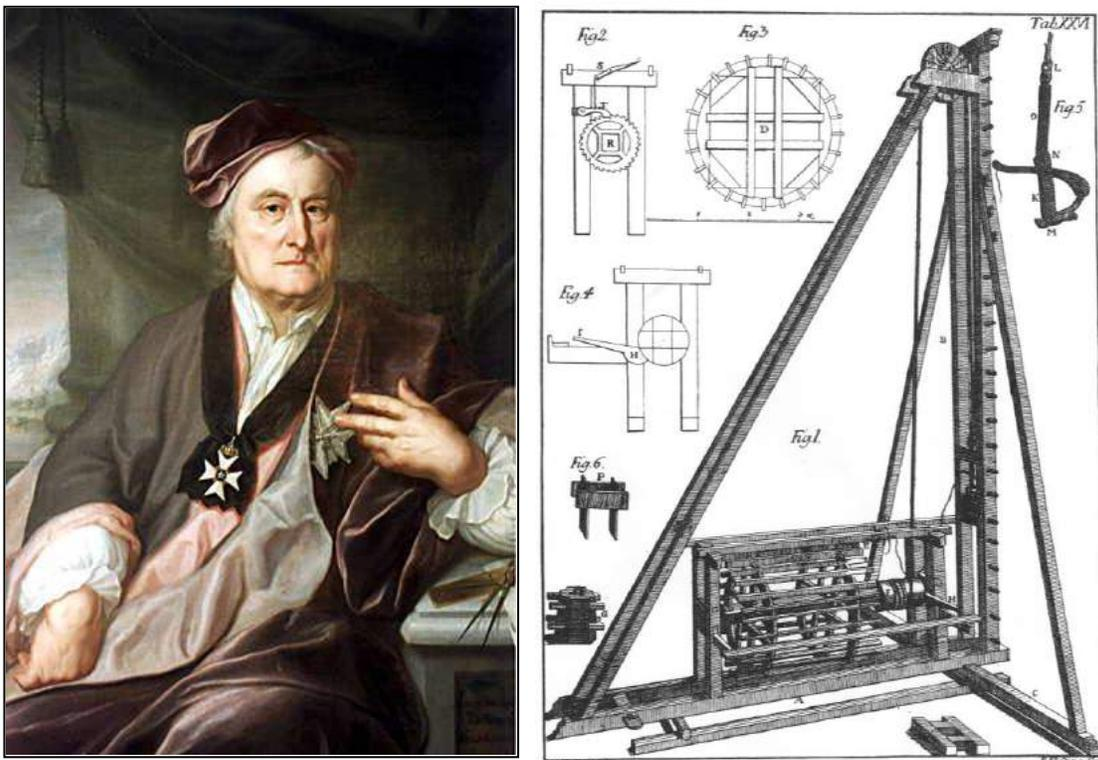
**Fig. 2 Christopher Polhem (painting by J. H. Scheffel in 1741) and a piling rig designed by Polhem for the construction of the sluice and lock in Stockholm**
